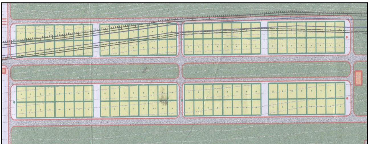
Figure 1.2-2 Positioning of chambers in the disposal modules
