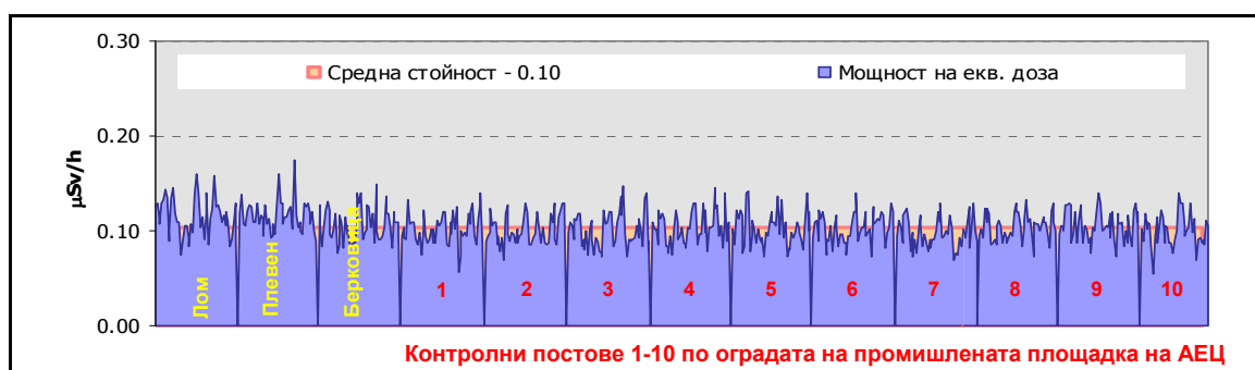
Figure 3.1-27 Power of the equivalent dose ( \mu\text{Sv/h} ) of gamma radiation in residential locations in H3 and the fence of Kozloduy NPP, 1996–2008
